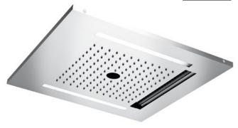
Note: Notes: connessioni | connections G1/2" / NPT - con telecomando e trasformatore per cromoterapia inclusi - with chromotherapy remote control and transformer included | telaio incasso e kit di connessione inclusi | built-in frame and connection kit included - tecnologia RGB con strisce led | RGB technology with led stripes | completamente ispezionabile | completely inspectionable include kit fissaggio security fix per soffioni pesanti | includes security fix kit for heavy shower heads
